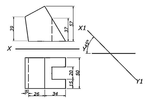
7. Figure below shows a block in orthographic projection. Reconstruct it in isometric projection.
