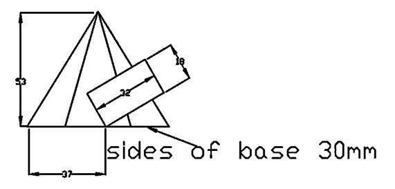
6. Figure below shows a block; construct its auxiliary front elevation on X1 - Y1.
